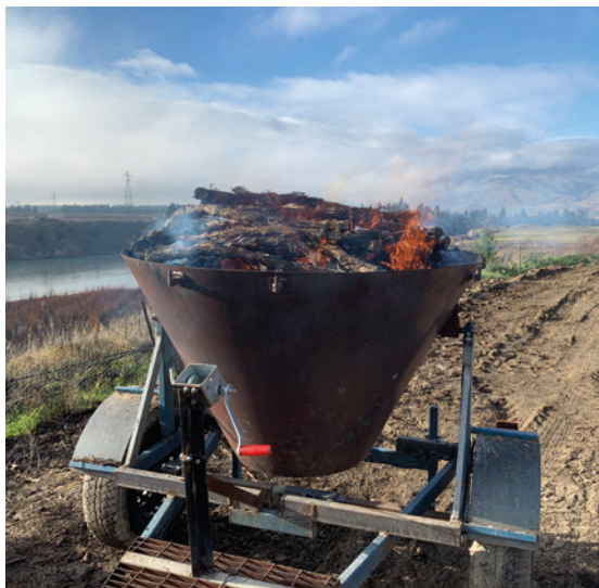
Biochar produces a clean burn with little or no smoke when using a specially designed kiln at Mt Difficulty in Central Otago. Photo: James Dicey
